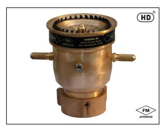
Clean the nozzle and reassemble. While re-assembling the nozzle or as a normal preventive maintenance, water proof lubricant must be used on seal and moving parts for smooth operation. The nozzle must be operated periodically under full flow straight stream and for fog pattern.
